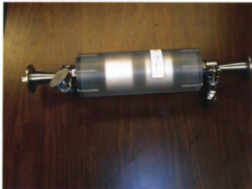
PLATE 1 Co-field flow PEF treatment chambers for benchtop and pilot plant-scale PEF system using stainless steel electrodes (top), a PEF treatment chamber for pilot plant-scale PEF system using stainless steel electrodes (middle), a PEF treatment chamber for pilot plant-scale PEF system using boron carbide electrodes (bottom).
